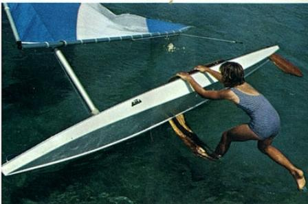
**SAFETY** is built in. Foam flotation, bonded to the inside of each Fibreglas hull, makes them unsinkable. In the event of a capsize, righting is easy. For added safety, the wearing of approved lifesaving equipment is recommended.
